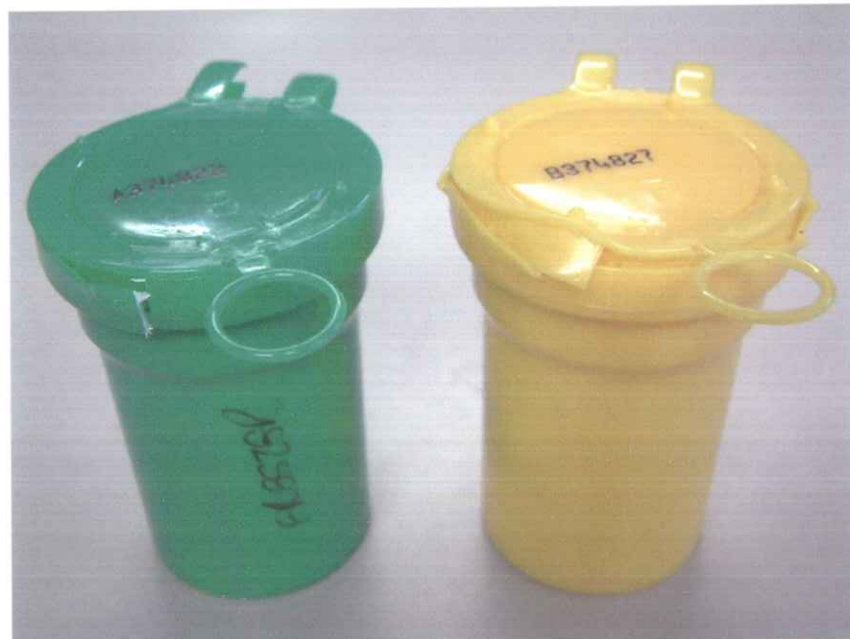
Figure 3 – Tamper evidence caused by leverage of the canisters lid at -18^{\circ}\text{C} (left) and 55^{\circ}\text{C} (right)
