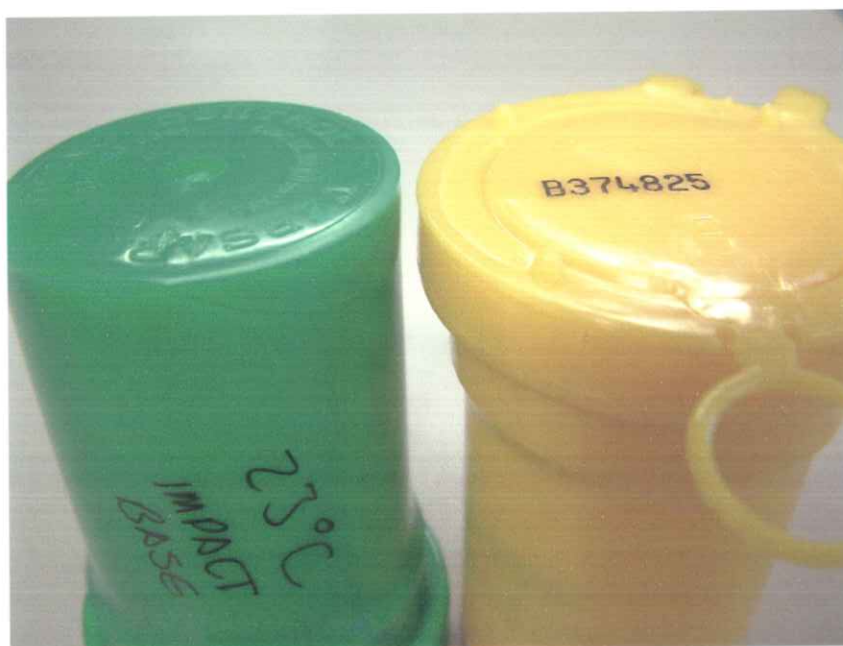
Figure 2 – Cracked canisters caused by impact damage
