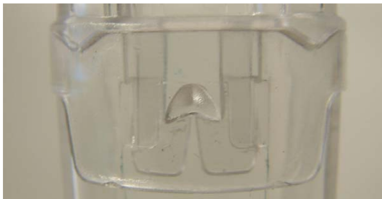
Figure 4 – Interlocking features covered by the lid
