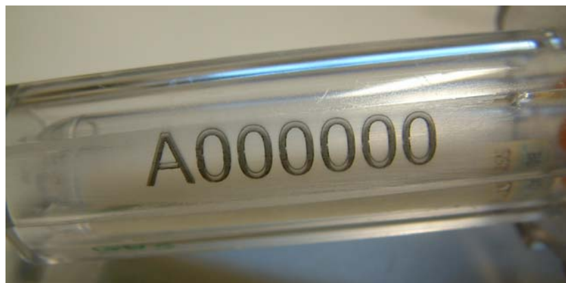
Figure 5 – Serial number remains visible after abrasion
