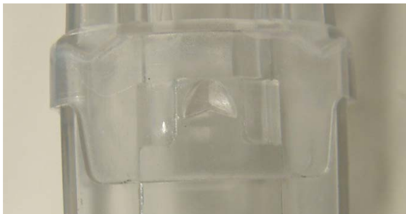
Figure 7 – Reclosed lid bonded to the canister body without repairing/replacing the latch features
