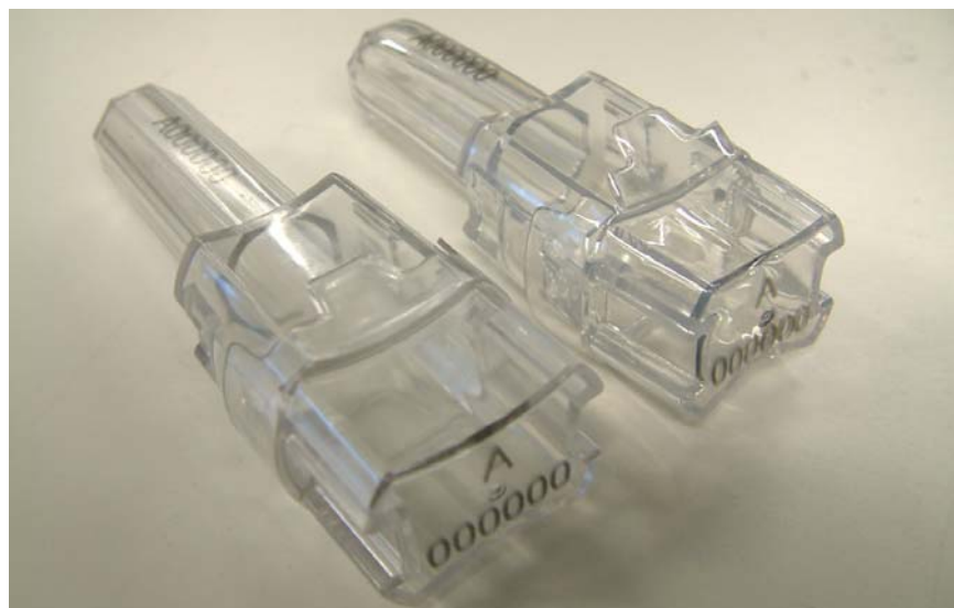
Figure 16 – Comparison of canister appearance before (left) and after heating to 90°C (right)
