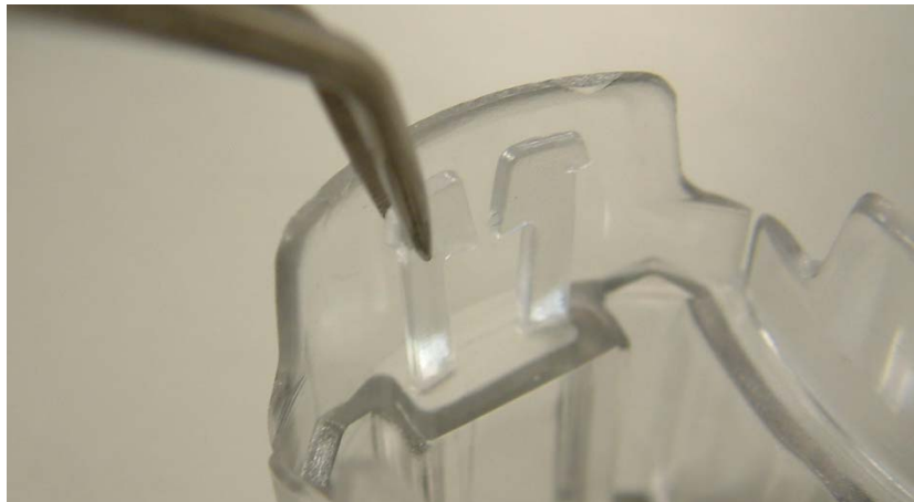
Figure 6 – Reattaching the broken latches, some whitening is visible in the bonded area
