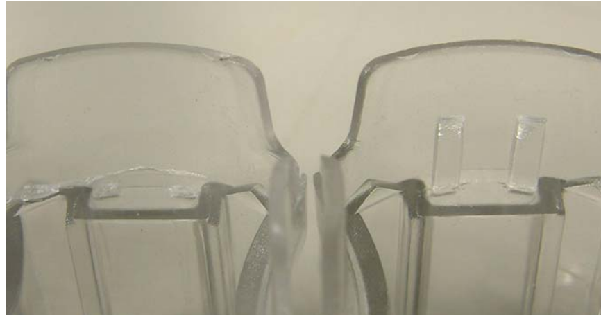
Figure 15 – Typical latch damage after cold and ambient opening (left) and hot opening (right)
