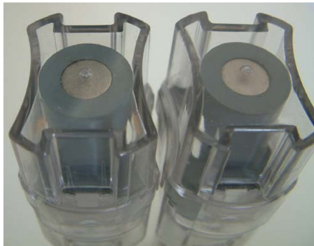
Figure 11 – Comparison of tampered and repaired canister (left), and untampered canister (right)
