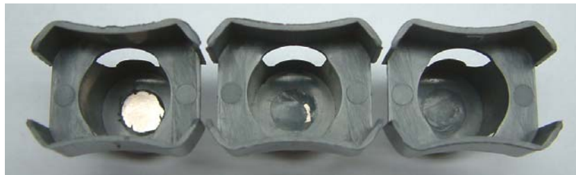
Figure 14 – Variation in metal insert embedment in caps
